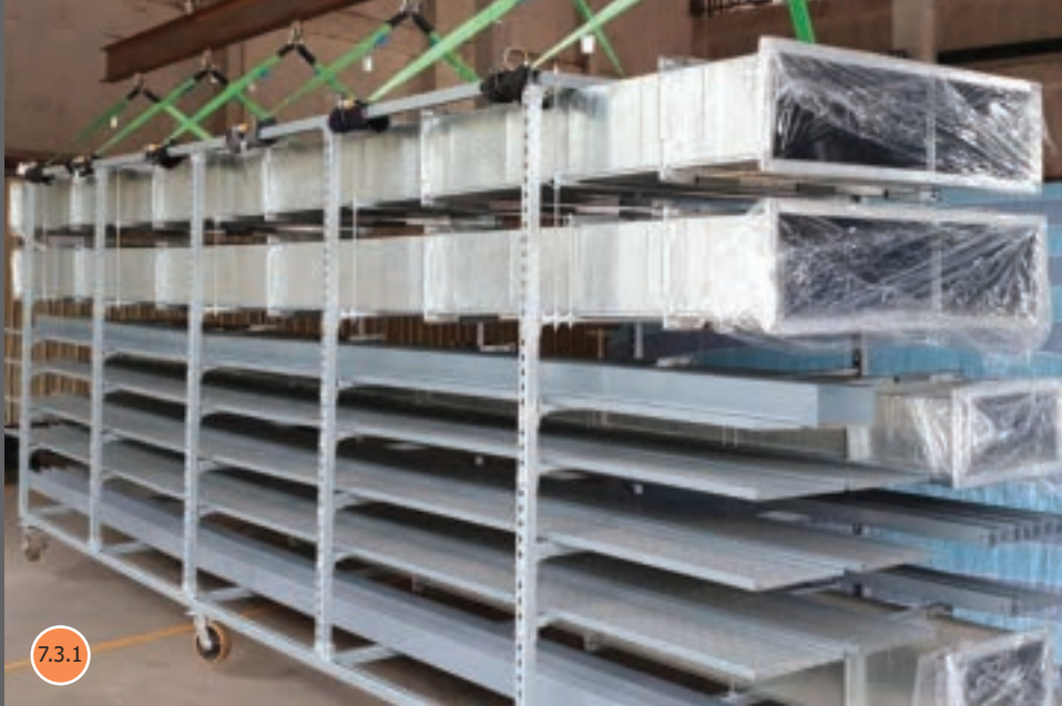
FIGURE 7.3.1 Horizontal module completed in factory and ready to be delivered to site
